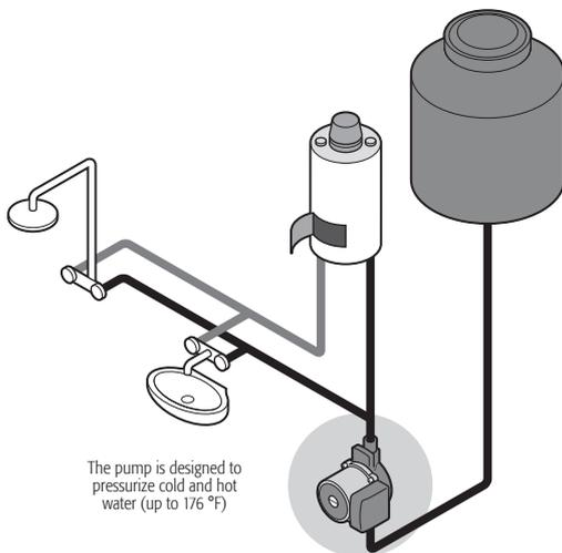
The pump is designed to pressurize cold and hot water (up to 176 °F)
